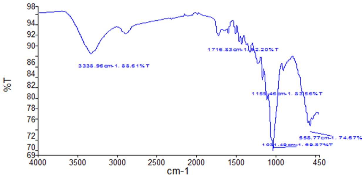
**Figure 2: Spectrum of the acetic anhydride modified *Celtis mildbraedii* wood samples**
